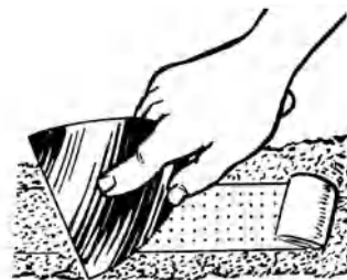
perforated tape covering a joint
