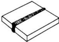
welded butt joint
