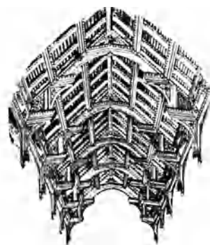
hammer-beam roof
