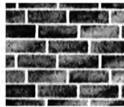
raking stretcher bond
