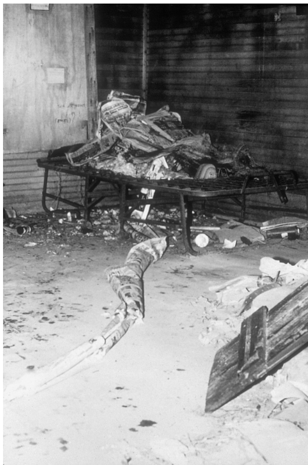
FIGURE A.6B Material used to make a fire trail, and debris piled in the corner of a room to ensure an intense fire.
