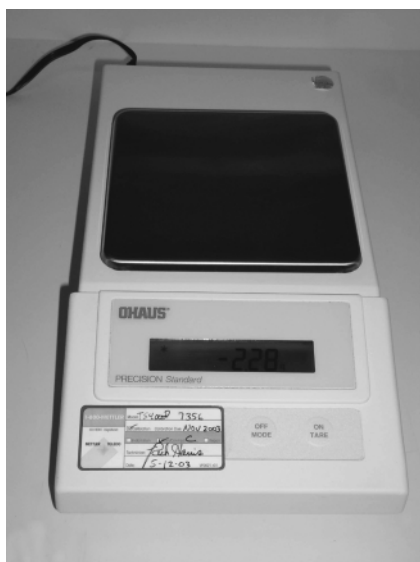
FIGURE A.3 Analytical balances used for measuring reagents, dry chemicals, and for measuring the accuracy of manual pipettes (the amount of fluid dispensed).
