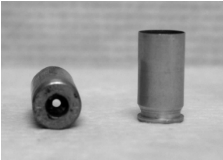
FIGURE C.3 Firearm cartridge in which the primer compound is contained in a centrally positioned primer cap.
