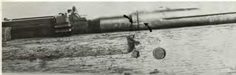
The two arrows point at the two marks known as witness marks which must coincide as shown for proper alignment of sights and headspace.
