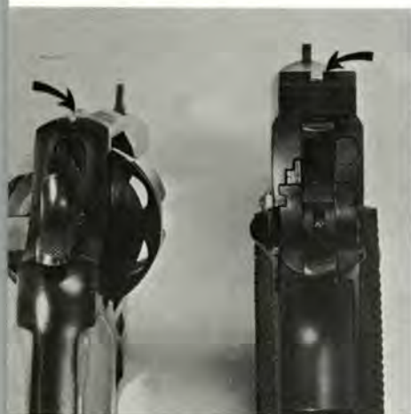
At left is double action revolver with non-adjustable sights. At right, the fully adjustable rear sight of a 45 ACP match gun.
