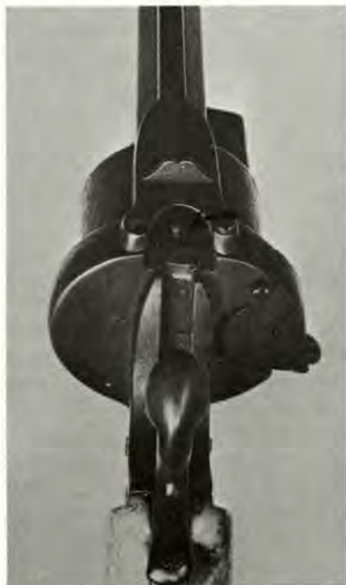
Belgian pinfire revolver. Arrow points to pinfire mechanism of cartridge in gun's chamber.
