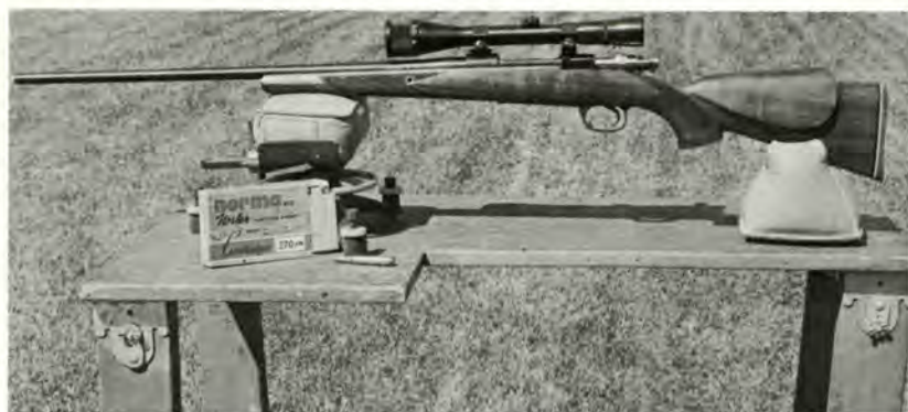
A metal pedestal rest with fitting sand bag for forend and buttstock is best for sighting-in. The same rest equipment is used in benchrest matches.
