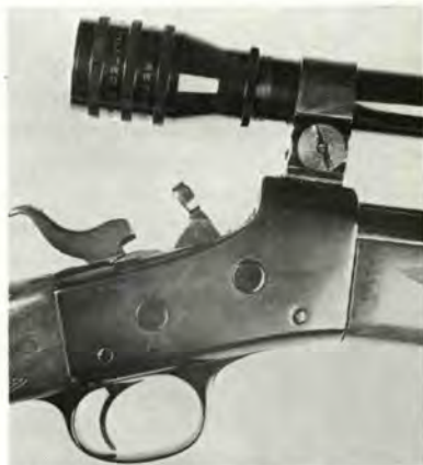
This Remington Rolling Block action was equipped with new barrel and stock. Note high scope base which is needed so that there is access to hammer and rolling block.
