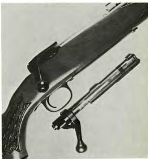
Above, bolt in rifle has been turned down by means of the bolt handle, gun is locked and cocked. Below, typical bolt with extractor near bolt face.
