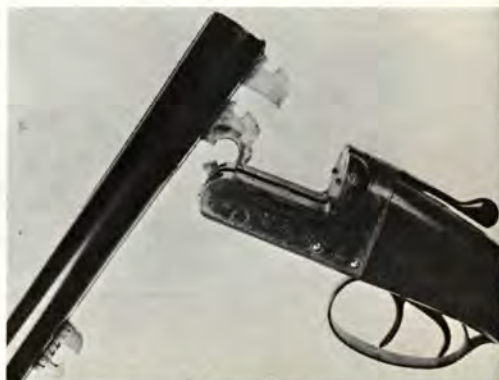
Typical bar of side-by-side English shotgun.
