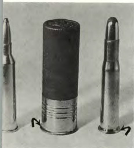
Semi-rimmed 225 Winchester at left, the rim of a shotshell, and the rimmed 30-30 round. Arrow indicates rim.
