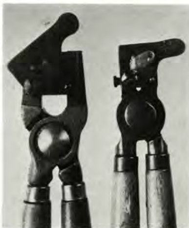
Mold at left shows sprue cutter moved up, mold at right shows cutter in place with sprue right after casting.
