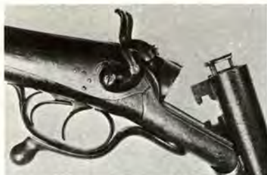
Old side-by-side top-break with underlever opening system. Lever fits below trigger guard, swings to right to permit opening of gun.
