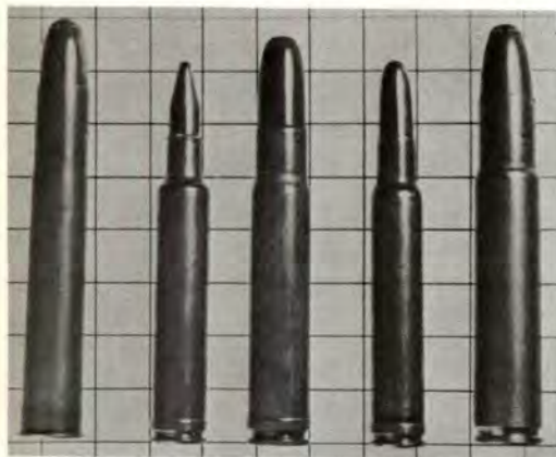
Magnum cartridges come in all shapes and sizes. The one at the left is rimmed, the three center ones are in belted cases, far right is a wildcat magnum without belt.
