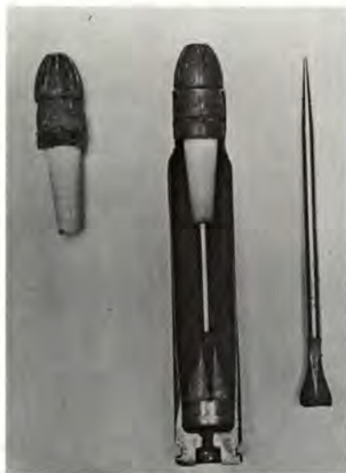
Sectioned XM 144 shows sabot and flechette in case.
