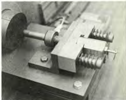
Pressure barrel in special firing device shows how strain gage is attached to barrel.
