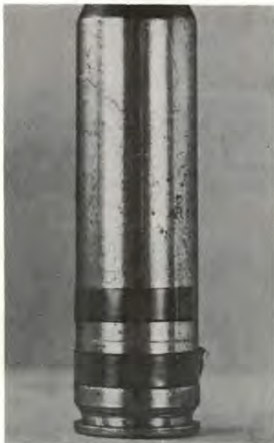
Fine, hairline crack just above belt of 350 Remington Magnum case indicates either excessive pressures or too frequent reloadings with max or near max loads.
