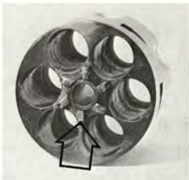
Arrow points to ratchet on rear of a revolver cylinder.
