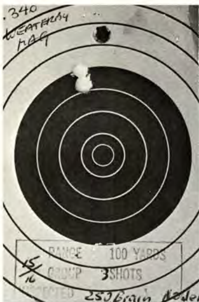
A 3 shot group at 100 yards measured only 15/16" from 340 Weatherby Magnum with 250 gr. Nosler bullets. Size of group, not location, is important when considering accuracy.
