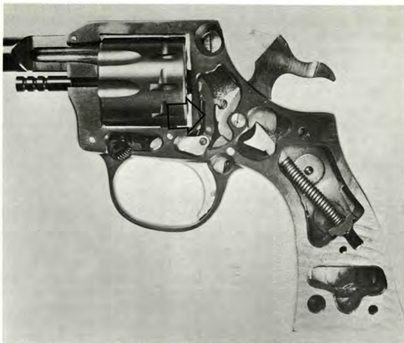
Model shows relationship of hand (arrow) with hammer, ratchet of cylinder, and trigger group.
