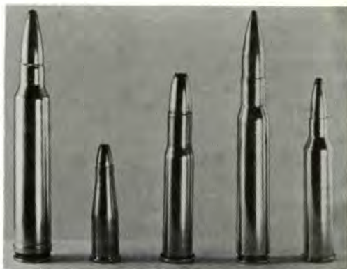
Left to right: Belted 375 round, bottleneck 22 Jet, rimmed 30-30, a rimless 30-06, and a semi-rimmed 225 Winchester.
