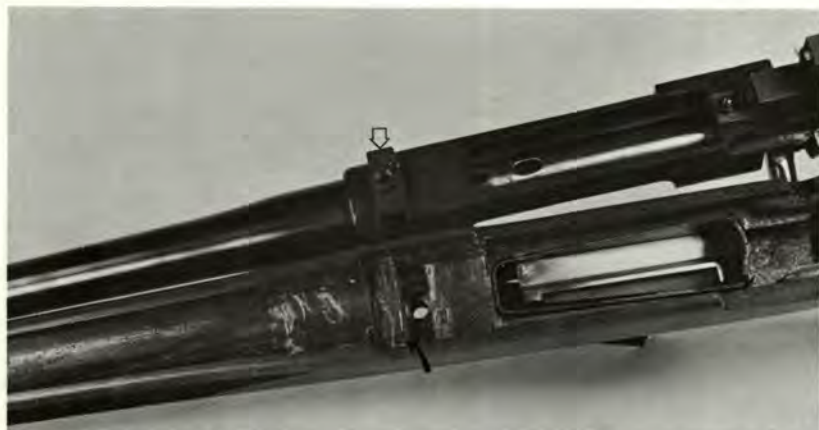
Arrow on barreled action indicates the recoil lug that fits into the abutment in stock. Arrow on stock indicates recoil shoulder in stock which, on this stock, has been glassbedded.
