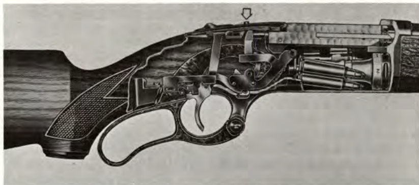
Savage Model 99 with rotating magazine.
