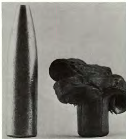
Bullet at left weighs 250 gr., was loaded for a wildcat rifle, the 338-06. Bullet at right was recovered from record moose, shows excellent expansion and better than 90 per cent weight retention.
