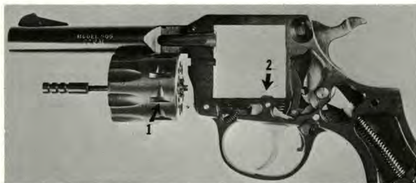
Cylinder stop notch (1) is engaged by cylinder stop (2) so that cylinder indexes properly.
