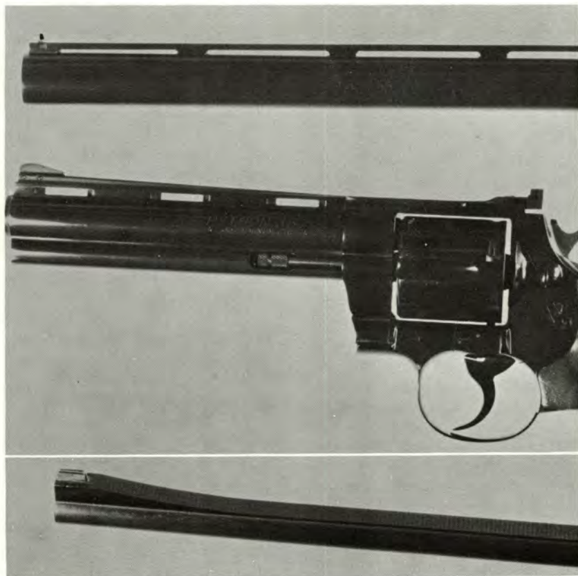
Ribs on three types of guns. Top to bottom: Ventilated ribs on a single barrel shotgun and on a Colt's 357 Magnum Python. Below, a solid rib on a sporting rifle.
