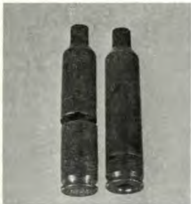
Complete separation at left, partial at right. Courtesy Shooting Times magazine.
