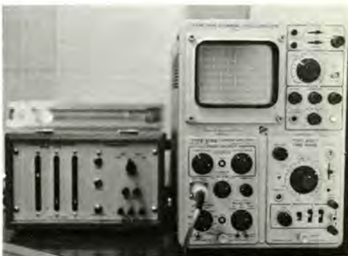
Equipment used to obtain velocity and pressure readings at the same time.
