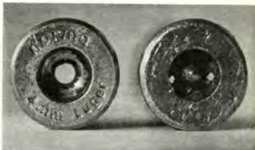
Case at left is for Boxer or American primer; case at right is suitable for the Berdan primer.
