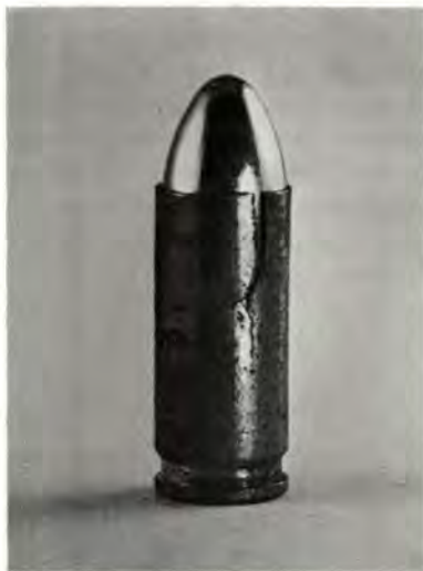
Season cracking of brass case.
