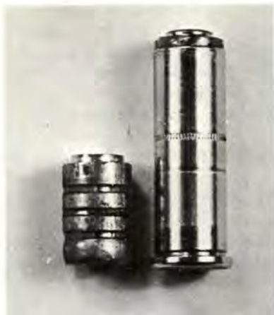
The wadcutter bullet, a cast lead bullet for the 38 Special match load usually weighs around 148 gr., contains three grease or lubrication grooves and is seated in the manner shown at right.
