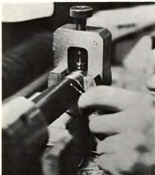
Gas check and crusher have been seated, and piston of crusher gage system is about to be set in place.
