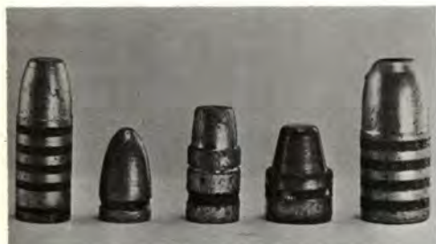
Many styles, shapes, and sizes of cast bullets can be made by the handloader. Dark bands are grease grooves.
