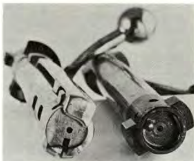
Bolt from Mauser M98 at left, and recessed bolt face of modern magnum rifle.
