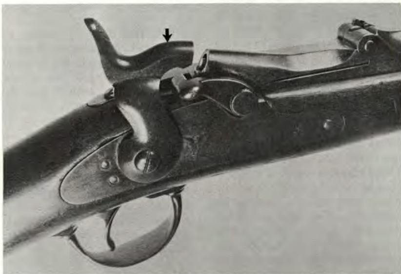
Sidehammer on the Springfield Trap Door 45-70.
