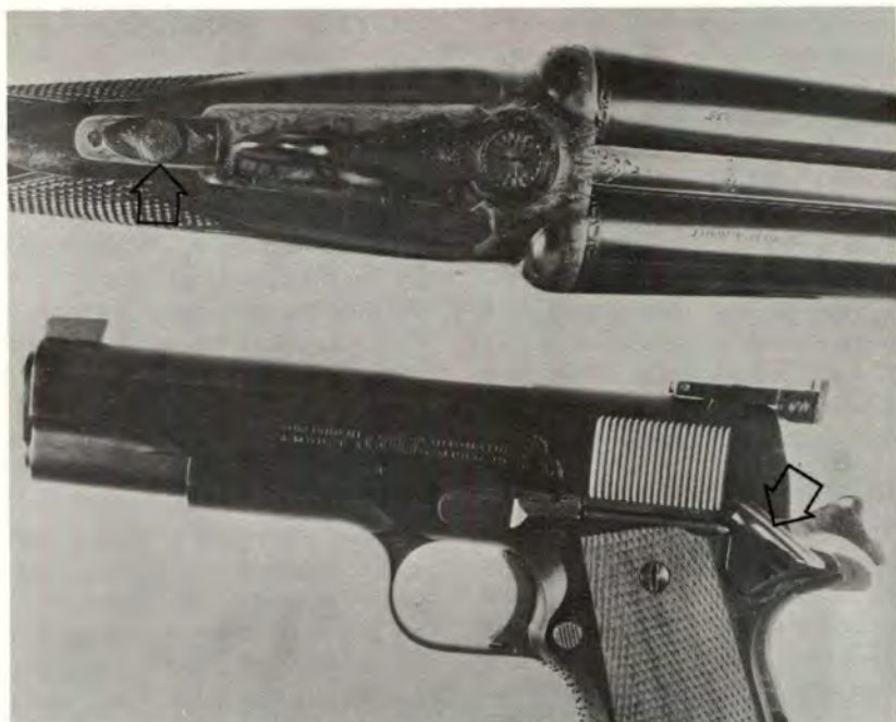
Sliding top-tang safety of a side-by-side shotgun and the slide safety of a 45 ACP.
