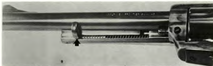
Coil spring on rod ejector of single action revolver is clearly visible. By pushing on finger rest (arrow), the rod ejector is moved to the rear so that fired case can be removed from chamber of cylinder.
