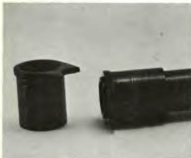
Barrel bushing on 45 ACP.
