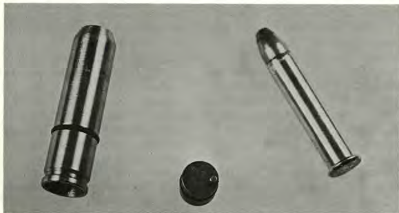
This auxiliary cartridge converts a centerfire rifle into one that fires a rimfire cartridge. Cartridge is inserted into body of auxiliary cartridge, then plug in center is seated in base of auxiliary cartridge.
