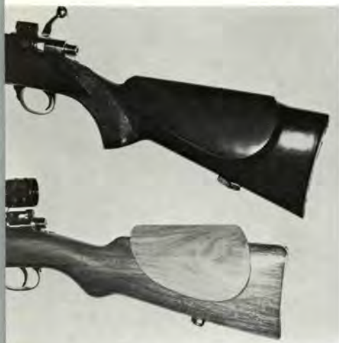
Dark stock shows cheekpiece that is incorporated into stock design; below, a cheekpiece that can be attached and shaped after stock has been finished.
