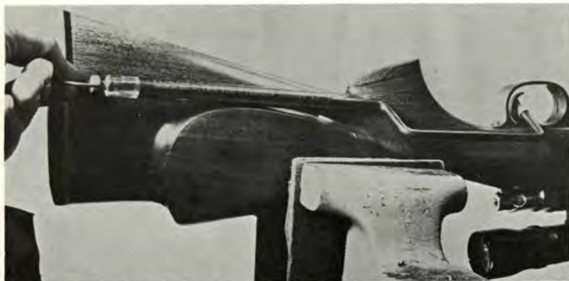
Shown is a spring trigger pull scale; for match use a rod with specific weights attached is used. Before using, ascertain that the gun does not contain a live round, either in chamber or magazine.
