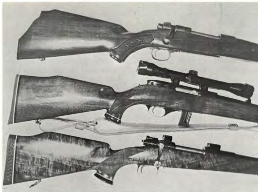
Impressed checkering at top; center, French or skipline checkering; bottom, fine-line checkering with 30 lines to the inch.
