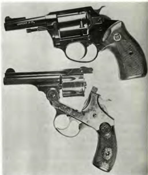
A solid frame 38 Spl. revolver with a hinged frame revolver below.
