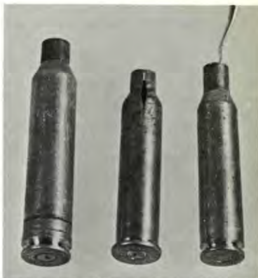
Incipient case head rupture at left; center: Rupture due to excessive cold working of brass; at right and barely visible, a case mouth fissure at pointer due to too frequent reloading and cold working of case mouth.
