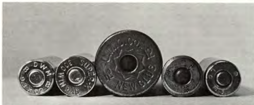
Markings on case head can tell where ammunition was made, what caliber, and in military rounds, when.
