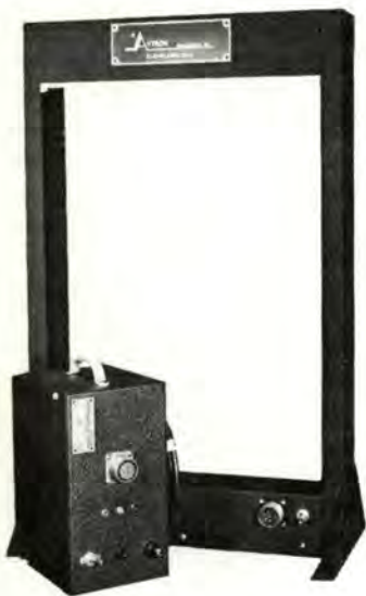
Avtron chronograph and Avtron photoelectric screen.
