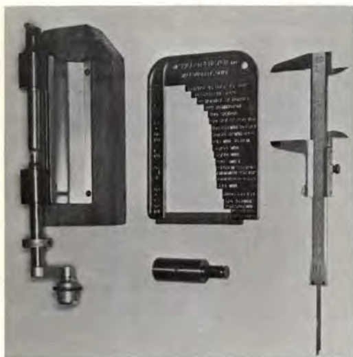
Case trimmer at left permits reducing case length after setting of trimming cutter stop. Center, top, a case length gage suitable for numerous calibers, below a case length gage for one caliber. At the right, a vernier caliper.
