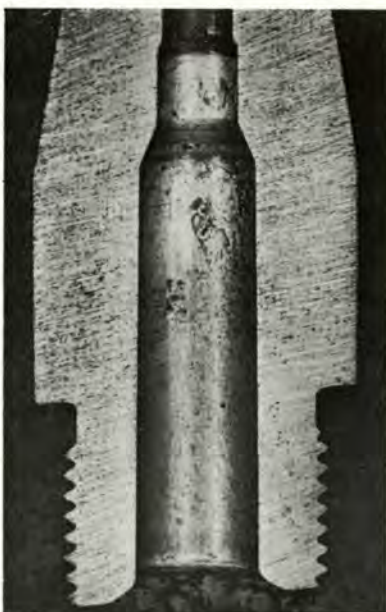
Corrosion due to high humidity in the chamber of M16.
