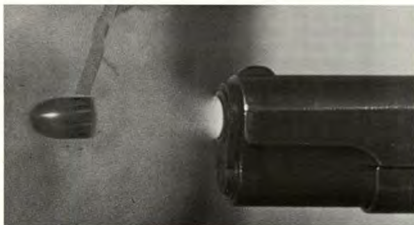
A bullet from a 45 ACP clearly shows the rifling marks or bullet engraving. Photo courtesy Shooting Times magazine.
